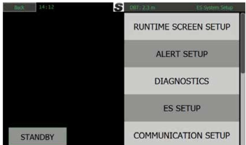
Additionally the “STANDBY” button is available to put system in standby for a period not in use. Will switch off the display and pinging.
