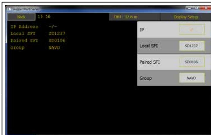
IP: The screen IP can be set up. recommended range is 172.16.1.X , but any private IP address is supported. The IP address must be unique for each unit. The mask is set to 255.255.255.0
