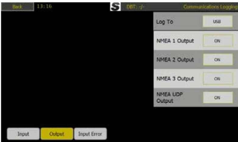
Setup for additional logging of NMEA and/or NMEA UDP to disk
