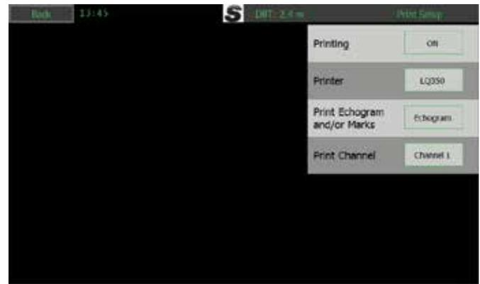
Select Printing “ON”, select the correct printer and channel.
